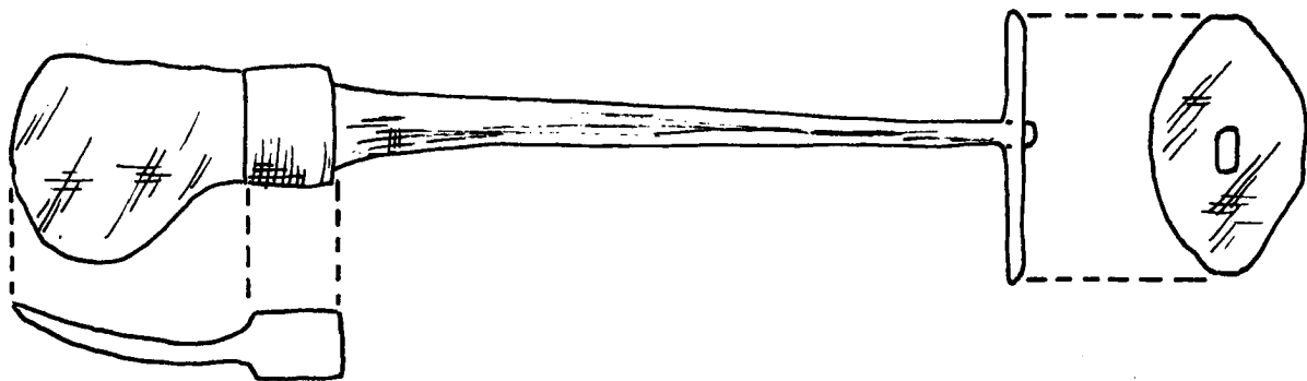
WELL WORN BLADE WITH RAT-TAILED TANG, POMMEL CAP AND UNGROOVED COLLAR REWORKED INTO A HAND GOUGE
